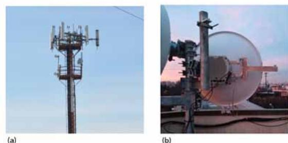
Figure 3 Test range comprising a typical 30 m high monopole for telecom backhauling (a) and three-foot EMBS prototype antenna (b)
